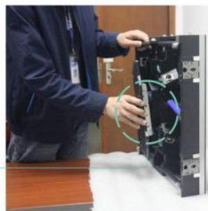
Modular designed core components enable fast replacement
